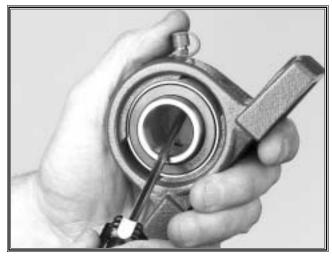
Figure 58. Bearing positioning for removal.
